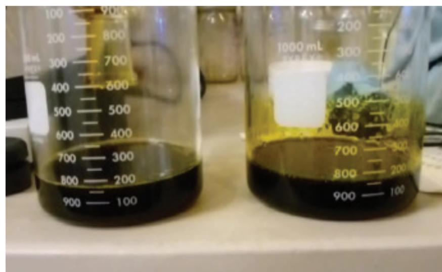
Figure 2. Refined THC oil extract: Left, from rotary evaporator; Right, from Rocket 4D Synergy evaporator.
