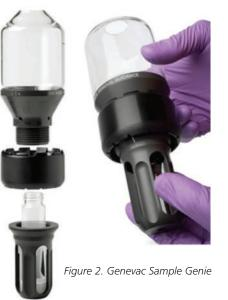
The Rocket Sample Genie flask system (Figure 2) enables samples to be dried directly into an appropriate vial of choice. Vials are attached to a 250ml capacity flask be means of a special adapter and support collar. Solvent in the flask is evaporated leaving the dried product in the vial which can then be detached. This eliminates time consuming sample transfer steps which can also reduce recovery.
