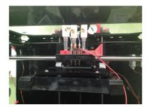
cells during the dispensing process. The bio-ink reservoirs were kept as close as possible to the valves in order to minimise the amount of time it would take to charge the system with bio-ink and to purge it at the end of the experiment. A USB microscope is also included to enable visual inspection of the target substrate
