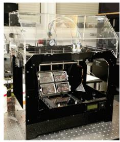
during the printing process. Due to the type of deposition system used, a direct line of sight view through the nozzle is not possible and therefore the USB microscope is mounted at an offset angle from the cell deposition system assemblies.
