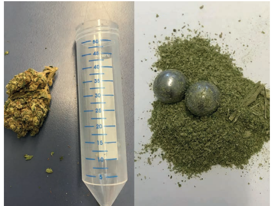
Figure 6. Flower buds before and after grinding in a 50 ml Falcon tube using the Mixer Mill MM 400.
