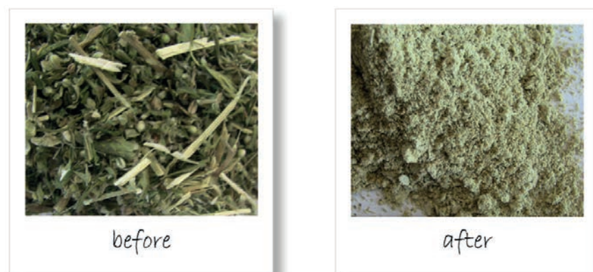
Figure 3. After pre-cutting in the SM 300 (left) the sample is pulverised to <0.5 mm in the ZM 300.
