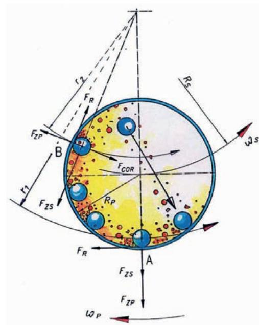
Figure 4. In the planetary ball mill, centrifugal and Coriolis forces permit
