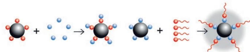
Figure 1. Neutralisation of charged particles by adding a buffer (electrostatic stabilisation, left) or by adding long-chained molecules (steric stabilisation, right)
