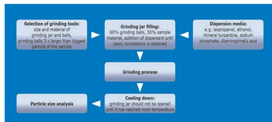
Figure 2. The steps of colloidal grinding
