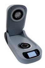
A further advantage of AwTherm is the removable measurement head, which means that the probe can be temperature calibrated or adjusted to achieve high precision.
