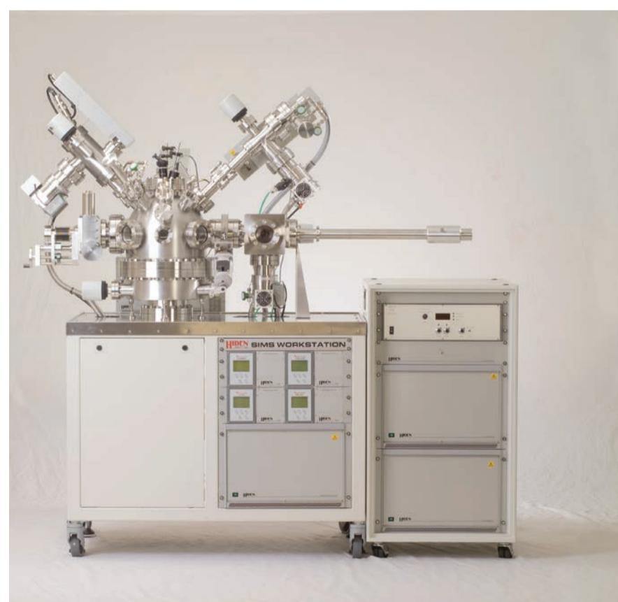
SIMS Workstation for thin film depth profiling
