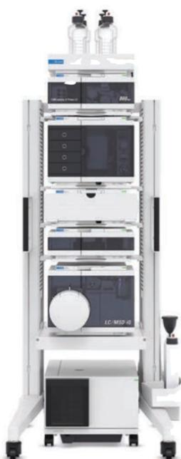
Figure 1. InfinityLab LC/MSD iQ.
