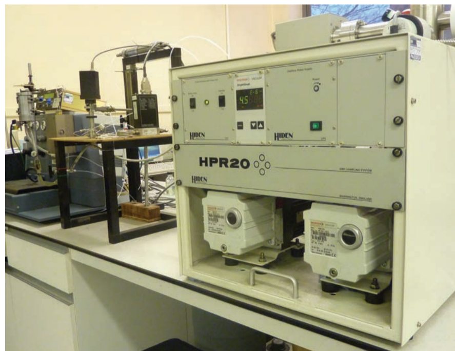
Figure 1: Flow adsorption calorimetry instrumentation. The flow-through Setaram DSC111 differential calorimeter is visible on the extreme left. The sample tube is held vertically in the stainless steel furnace. The automated gas sampling valve is visible on the platform in front of the calorimeter. The low-flow capillary interface to the Hiden HPR-20 Mass Spectrometer can be seen under the valve platform. The tube furnace alongside the calorimeter is for catalyst activation.
