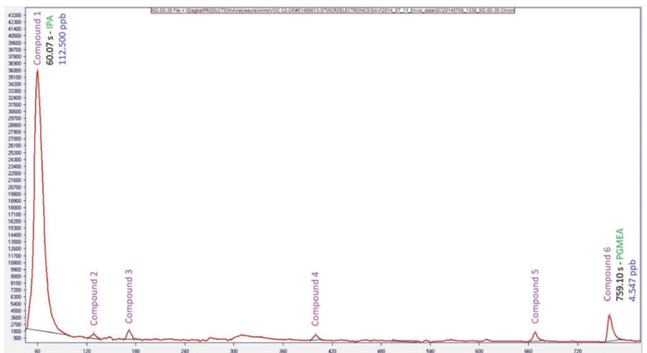
*Figure 1: GC chromatogram representing the automatic identification of IPA and PGMEA peaks respectively, the most representative VOCs monitored for semiconductor applications.*
