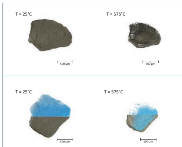
Untreated biomass particles (on the left) change their dimension with temperature (on the right) and showing their evolution when undergoing pyrolysis.
