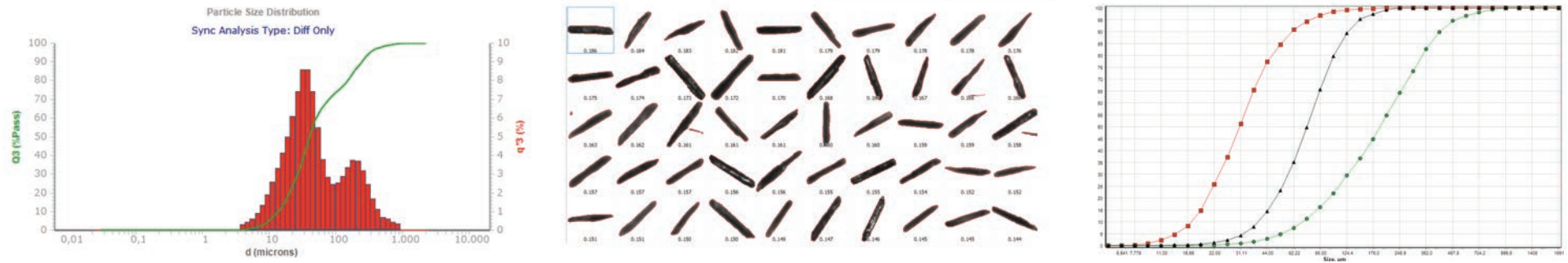
Figure 4. Analysis of needle-shaped crystals with laser diffraction results in a bimodal distribution (left) representing both width and length. With Image analysis, individual distributions for width and length can be measured (red and green curve on the right).
