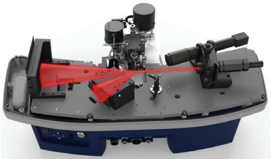
Figure 1. The SYNC analyser is a hybrid instrument that combines Laser Diffraction and Dynamic Image Analysis.
