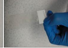
Figure 3. The Easylift coated slide. This image shows the slide viewed from the uncoated side, with the protective paper backing film on the underside of the transparent coating material.
