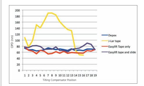
Figure 7. OPD measurements at different positions of a tilting compensator for an acrylic fibre held in depex, Easylift tape, Easylift tape and slide and J-Lar tape.
