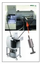
Figure 1. The EMPACT2 + RTS (top + bottom left) is a new mobile high-pressure freezer with an automated transfer attachment (Rapid Transfer System, RTS, top image) suitable for CLEM experiments. After insertion of the sample located at the tip (red circle) of the rapid loader (bottom right) into the RTS (red arrow), the RTS will automatically enclose the sample and transfer it into the high-pressure freezer where it will be cryo-fixed.
