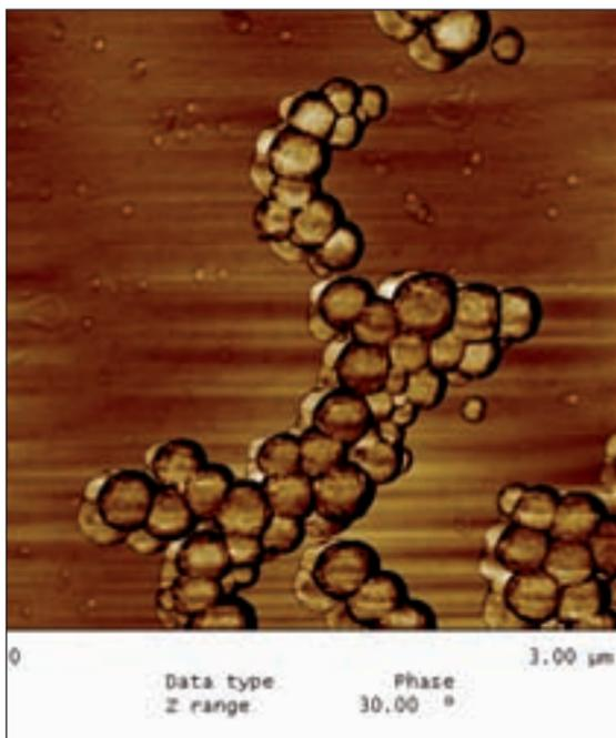
Particle size and structure of AMCO Clear® microspheres versus formazin
