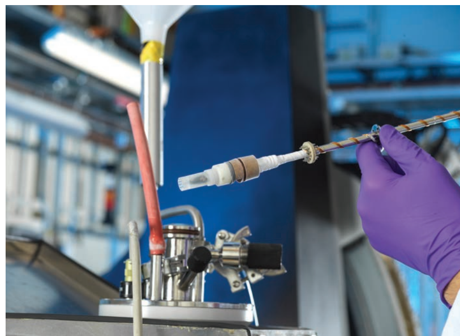
Demonstration of a sample containing uranium being studied and carefully loaded onto Diamond's I20-scanning beamline – Credit Diamond Light Source
