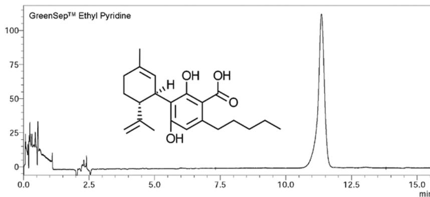
Figure 5: Cannabidiolic acid (CBDA) Chromatographed on GreenSep™ Ethyl pyridine. Operating conditions: column dimensions: 250 x 4.6mmID, 5µm particles, Total Flow: 3 mL/min, Mobile Phase: 0.3 mL/min methanol and 2.7 mL/min CO<sub>2</sub>, Back pressure: 150 bar, Column Temperature: 40°C, Detection: UV@254nm
