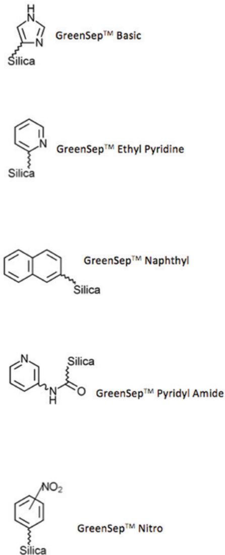
Figure 1: The Chemical Structures of SFC Optimised Stationary Phases Commercially Developed by ES Industries
