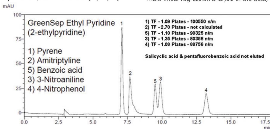
Figure 3: SFC Test Mixture Chromatographed on GreenSep™ Ethyl Pyridine. Operating conditions: column dimensions: 250 x 4.6mmID, 5µm particles, Total Flow: 3 mL/min, Mobile Phase: 0.3 mL/min methanol and 2.7 mL/min CO<sub>2</sub>, Back pressure: 150 bar, Column Temperature: 40°C, Detection: UV@254nm
