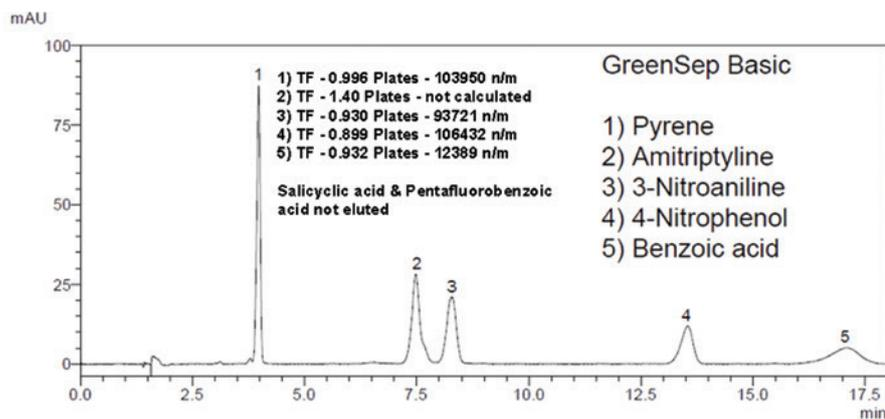
Figure 2: SFC Test Mixture Chromatographed on GreenSep™ Basic.
