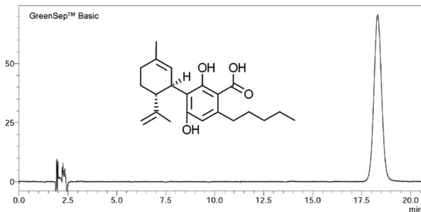
Figure 4: Cannabidiolic acid (CBDA) Chromatographed on GreenSep™ Basic. Operating conditions: column dimensions: 250 x 4.6mmID, 5µm particles, Total Flow: 3 mL/min, Mobile Phase: 0.3 mL/min methanol and 2.7 mL/min CO<sub>2</sub>, Back pressure: 150 bar, Column Temperature: 40 C, Detection: UV@254nm
