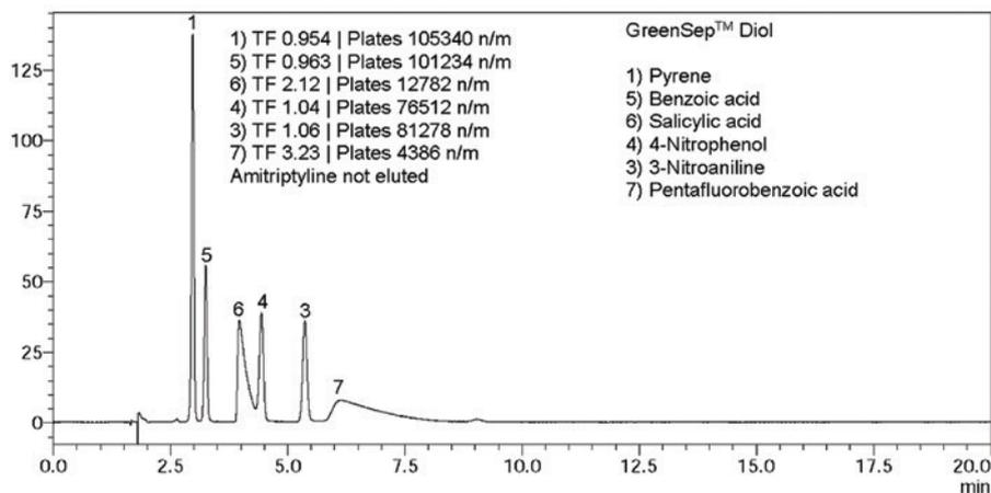
Figure 6: SFC Test Mixture Chromatographed on GreenSep™ Diol. Operating conditions: column dimensions: 250 x 4.6mmID, 5µm particles, Total Flow: 3 mL/min, Mobile Phase: 0.3 mL/min methanol and 2.7 mL/min CO<sub>2</sub>, Back pressure: 150 bar, Column Temperature: 40°C, Detection: UV@254nm
