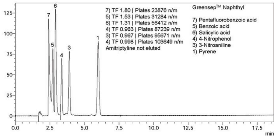
Figure 7: SFC Test Mixture Chromatographed on GreenSep™ Naphthyl. Operating conditions: column dimensions: 250 x 4.6mmID, 5µm particles, Total Flow: 3 mL/min, Mobile Phase: 0.3 mL/min methanol and 2.7 mL/min CO<sub>2</sub>, Back pressure: 150 bar, Column Temperature: 40°C, Detection: UV@254nm
