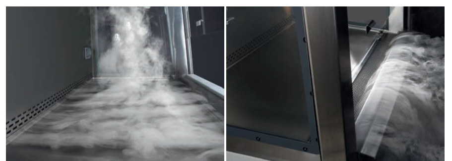
Figure 6: Class II BSC Airflow Dynamics.
