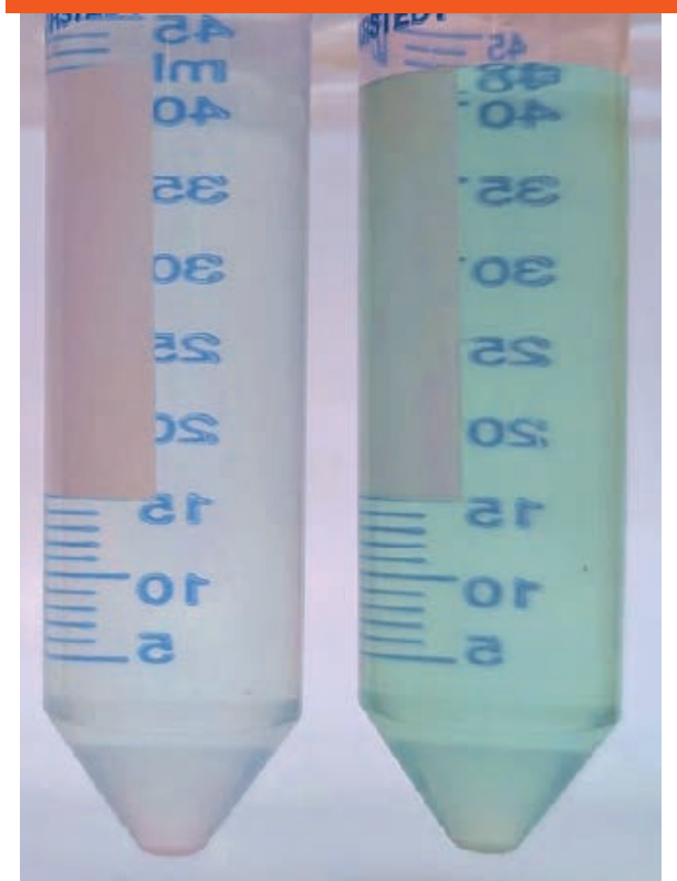
Figure 6: Digested solutions of black mass before leaching (left) and solid residue after leaching (right).
