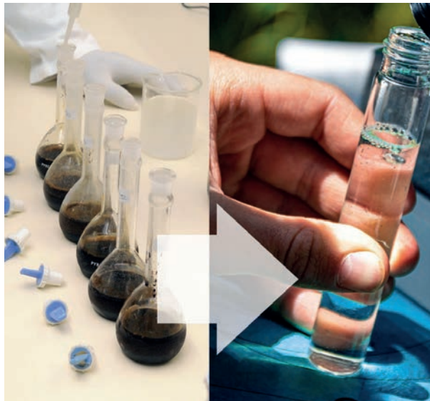
Figure 3: Example wastewater samples before and after nitric acid digestion according to DIN 15587-2.
