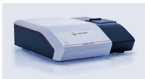
Figure 1: Litesizer DLS 501 particle size analyser employing dynamic light scattering (DLS).
