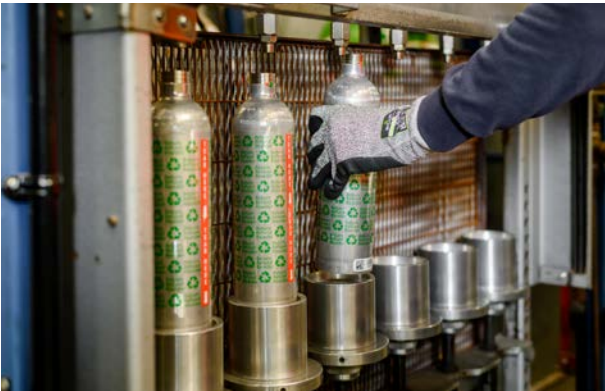
Closed loop refill system: after inspection and relabelling, the canisters are refilled for reuse.
