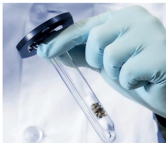
Figure 1: Catalyst sample in a quartz sample cell. Quartz wool is used to prevent migration of fine particles, especially when characterising powders.
