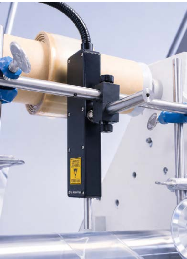
Figure 1: Raman probe integrated with the Univex film haul-off unit for non-contact Raman measurements of extruded and drawn PEEK film downstream of the cooling drums.
