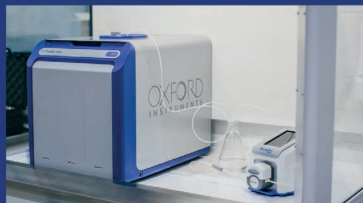
Figure 6: Schematic (above) and physical set-up (below) in a fume hood showing how flow chemistry is incorporated in the X-Pulse benchtop NMR instrument.
